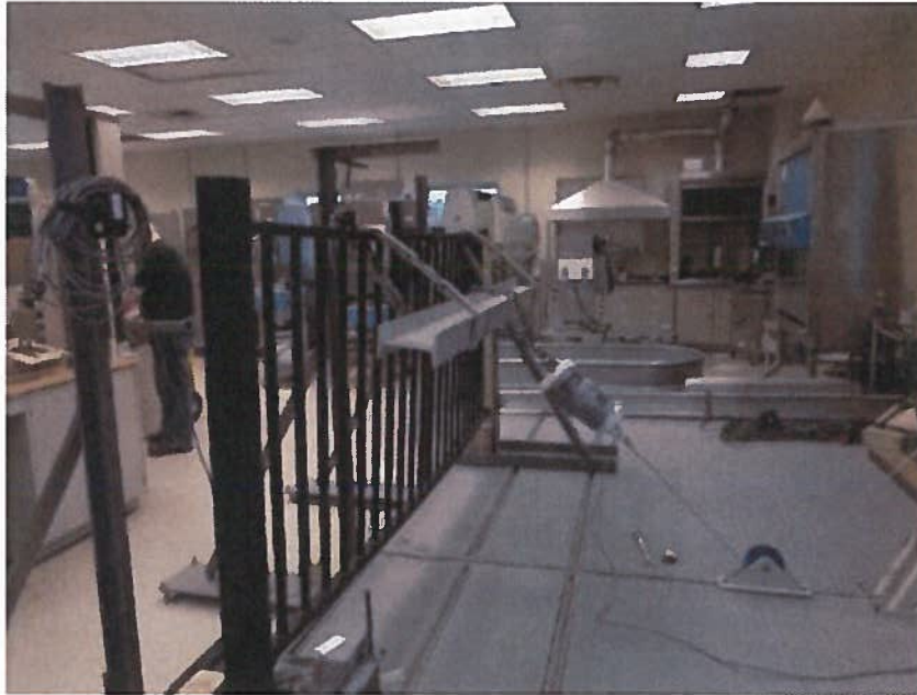
Photo No. 3 Uniform Load Test at 45° from Horizontal on Top Rail
