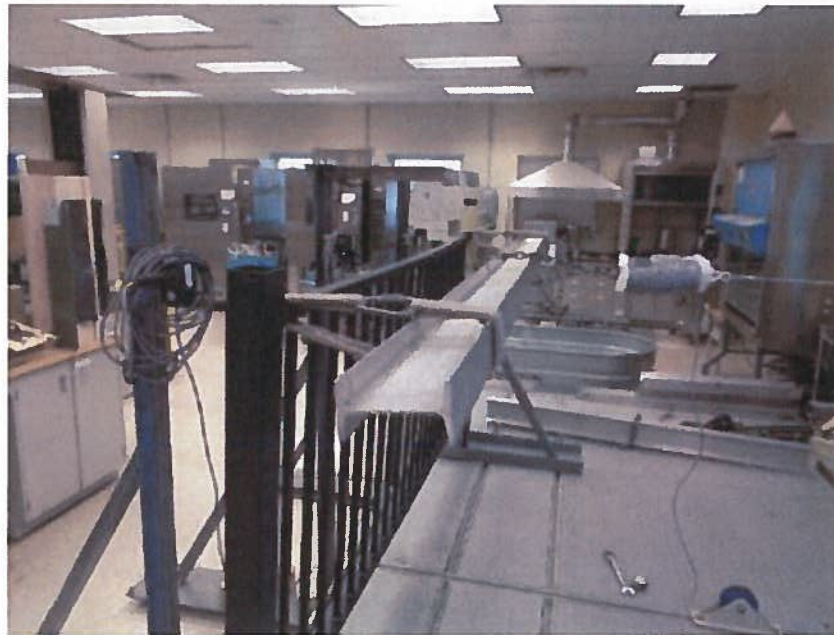
Photo No. 5 Concentrated Load Test at End of Top Rail (Brackets)
