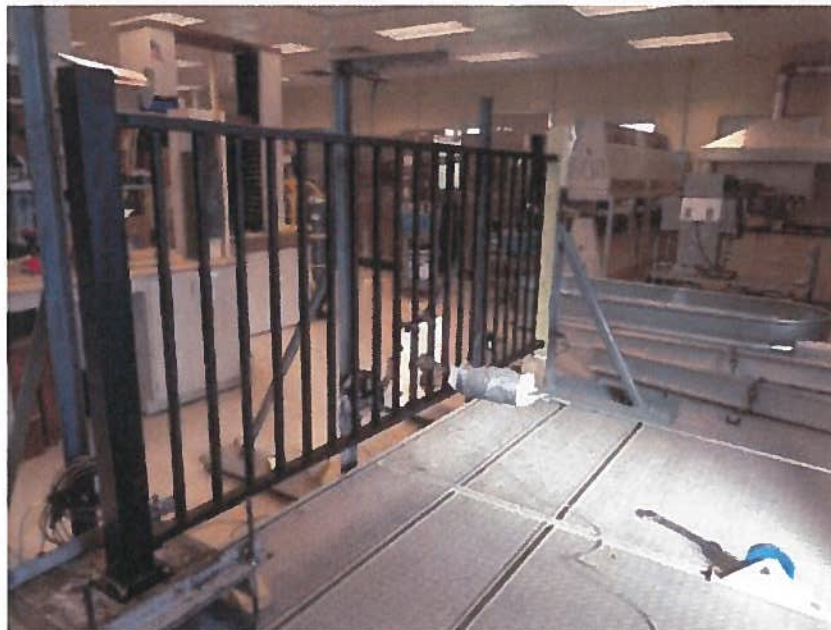
Photo No. 2 In-Fill Load Test at Bottom of Two Pickets
