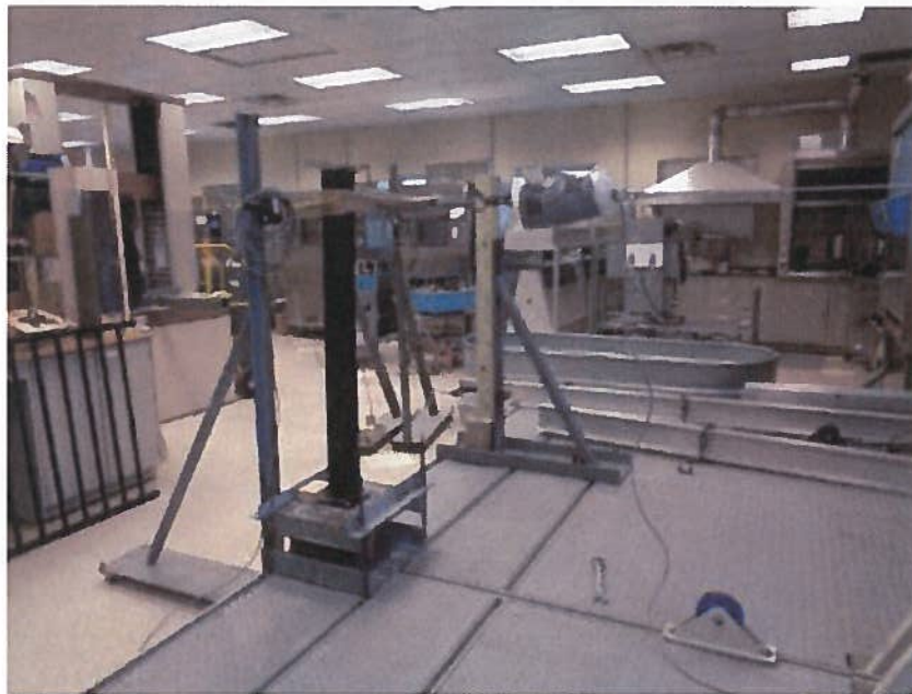
Photo No. 6 Concentrated Load Test at Top of Stand Alone Post Mount
